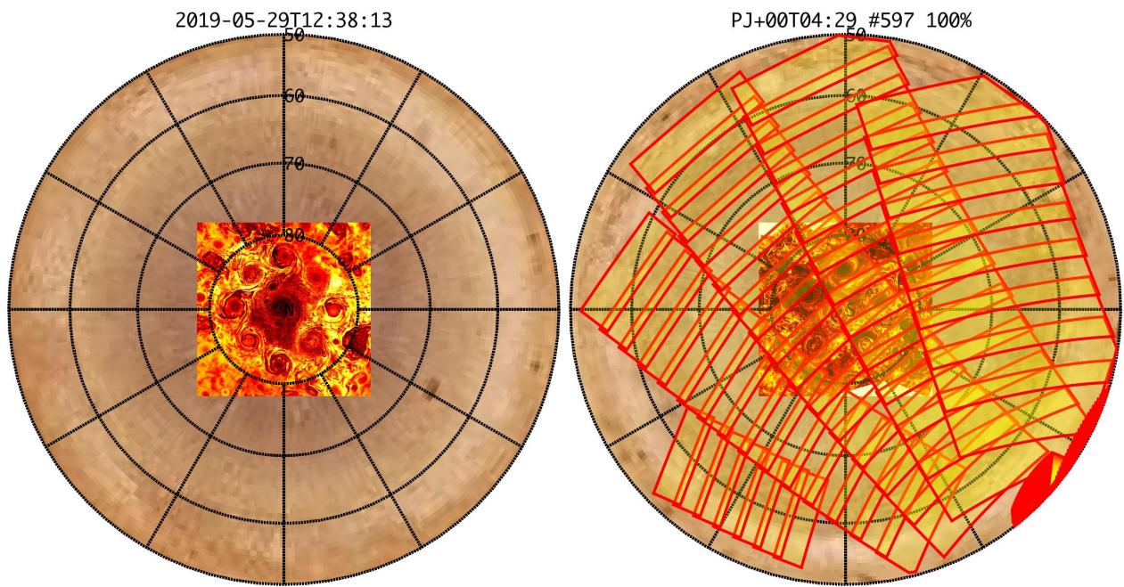
**Figure 1:** Simulation with JSPT (JIRAM Software Planning Tool), coverage of the South Pole with filter M. The overlapping yellow strips represent the predicted FOVs.
