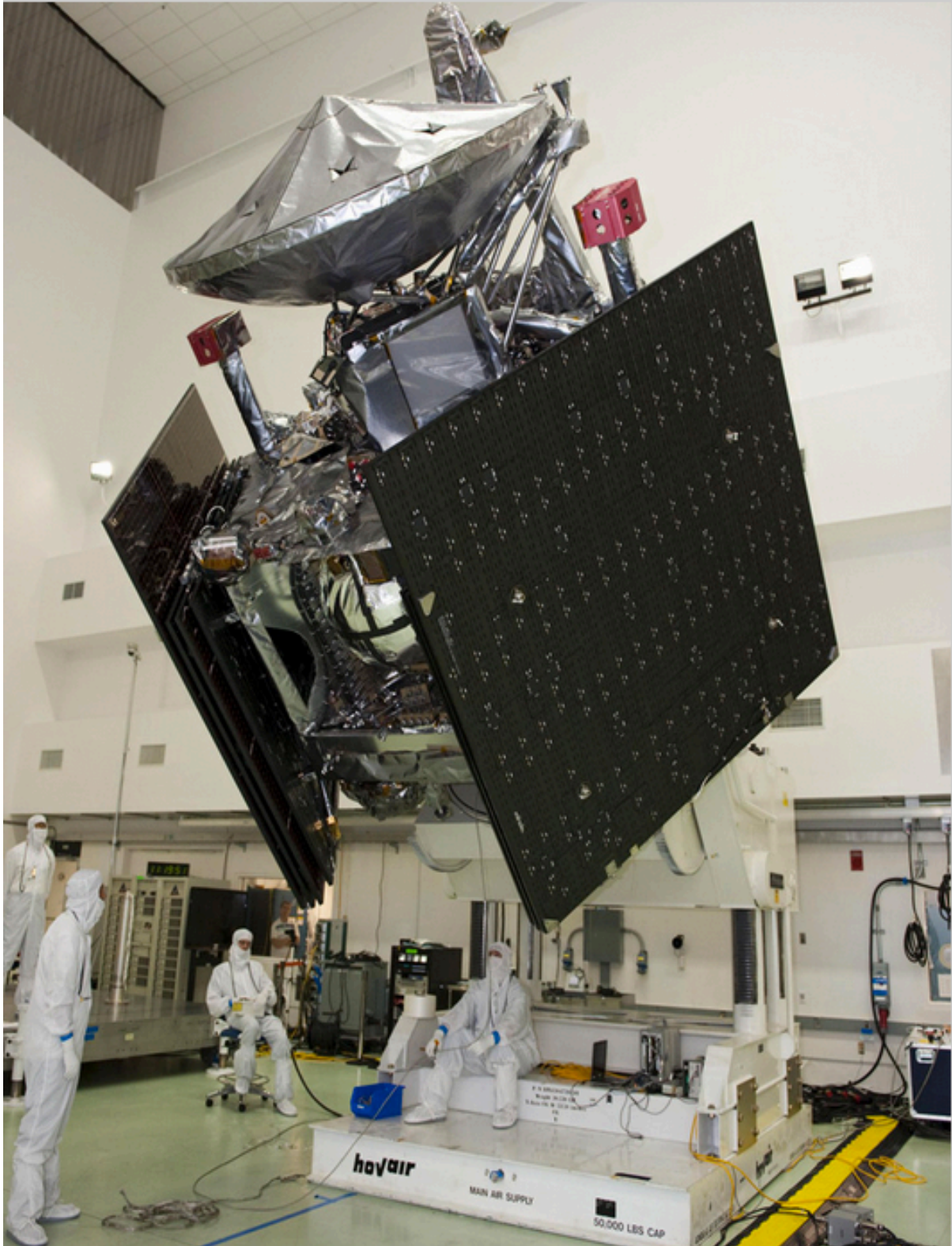
Figure 1. Testing of the Spacecraft. The large black areas are the folded solar cell arrays.
