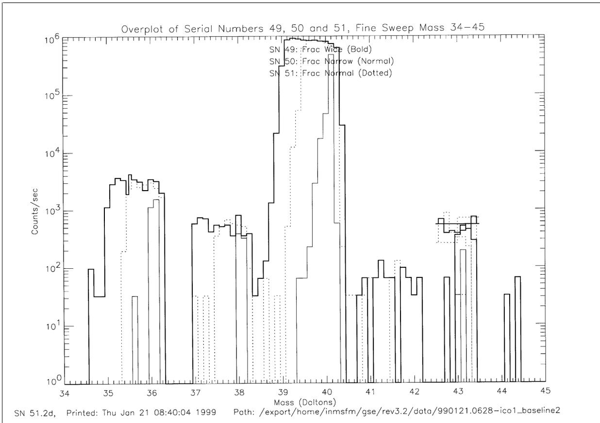
Figure 7.3 – Overplot of Fine Sweep with Peak Width Set Narrow, Normal and Wide
