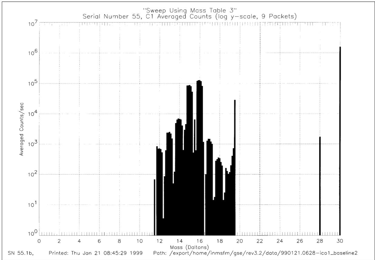
Figure 7.5 – Fine Sweep Using Mass Table 3
