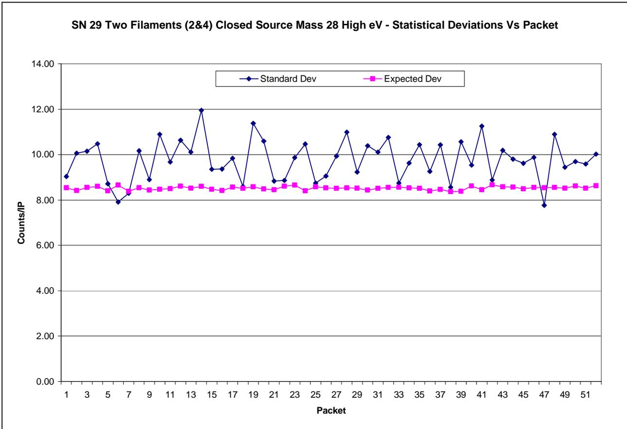
Figure 7.17 – SN 29 Comparison of Standard and Expected Deviation
