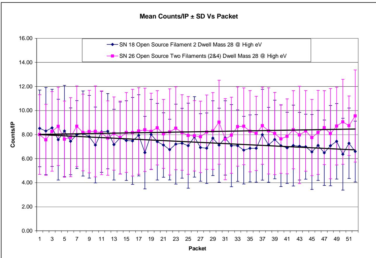
Figure 7.10 – SN 26 Counts/IP vs Packet with Standard Deviation
